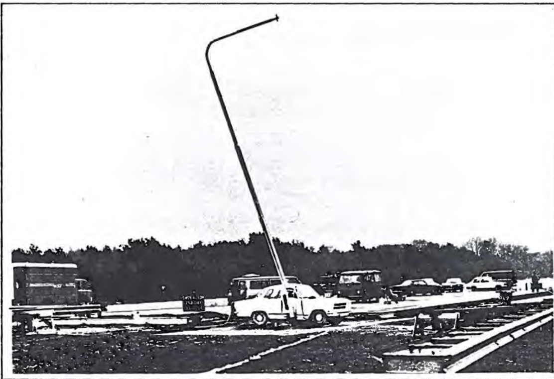
Figure 3.4. This 10 m aluminium column hit sideways-on in test series at 30 km/h gave acceptable vehicle decelerations. But it did not break; the vehicle came to a stop against it. The dent in the vehicle's flank exceeded the maximum.
