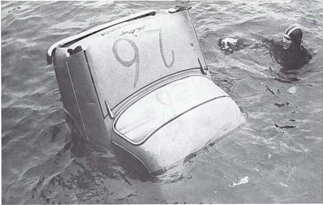
Figure 19. Cars with front engines almost always sink nose-downwards.
