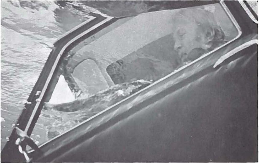
Figure 21. As the car sinks the air is forced to the highest part of the cabin so that one has a chance to fill one's lungs.
