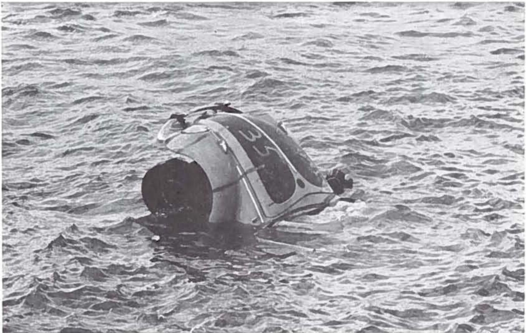
Figure 20. Rear-engined cars almost always sink tail-down.
