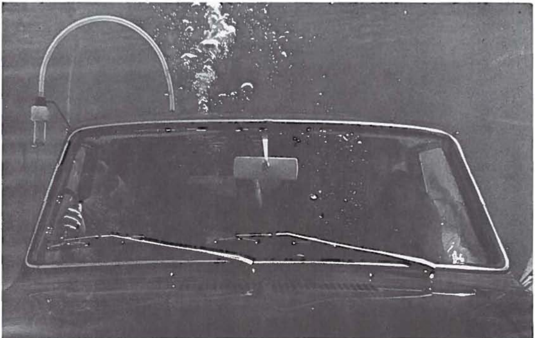
Figure 22. By the time the vehicle has come to rest on the bottom there will hardly ever be any air left in it.
