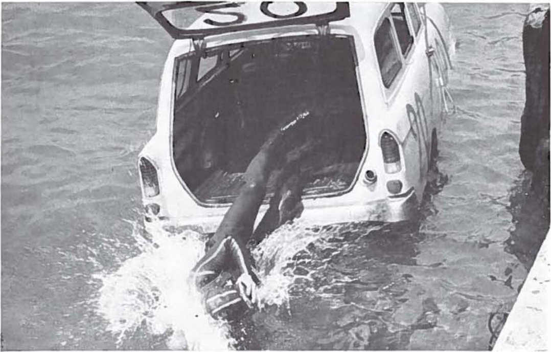
Figure 27. If a tailgate can be opened from the inside, it often proves to be a good escape route.
