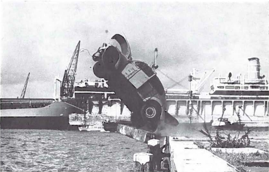
Figure 11. Often the vehicle collides with an obstacle just before crashing into the water, this may cause it to hit the water in strange positions.
