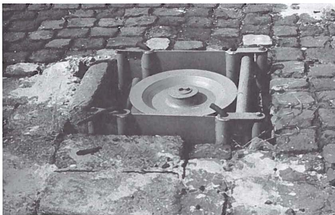
Figure 7. The winch cable was passed round a pulley and attached to the test vehicle.
