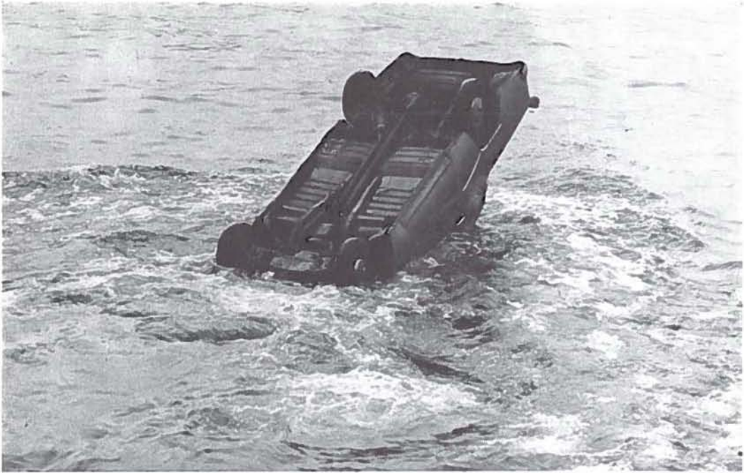
Figures 17 and 18. Most vehicles which hit the water upside down return first to an almost horizontal position before they sink.
