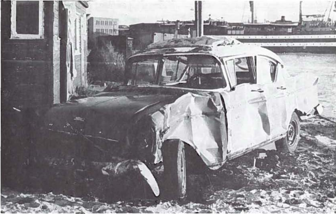
Figure 14. The result of hitting the water sideways: all the doors are jammed on the impact side.
