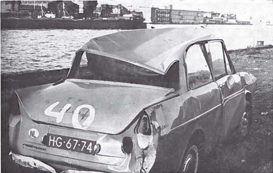
Figure 15. The cabin was badly pressed in because the vehicle landed on its roof.
