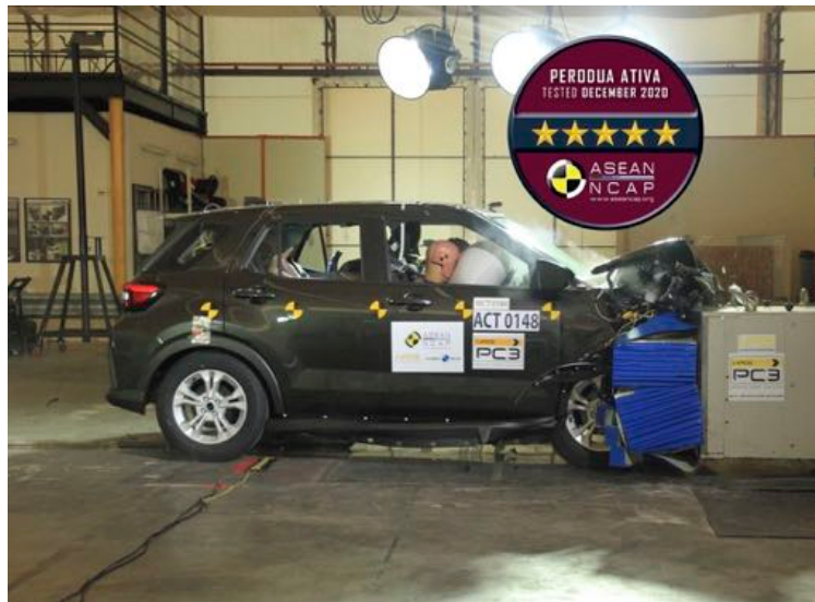
Figure 2.4.5. ASEAN NCAP crash test at PC3 Lab
