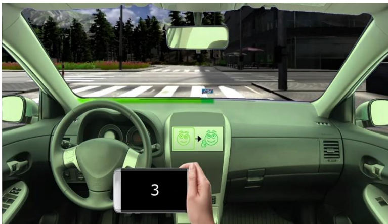
Figure 1. A screenshot from one of the videos included in the study (adapted from (Tinga et al., 2022)). The smiley face icons indicate the current automation level and the upcoming change, and the green progress bar indicates time remaining until the change. Participants monitored the driving while counting the number of times a “4” appeared on the mobile phone.
