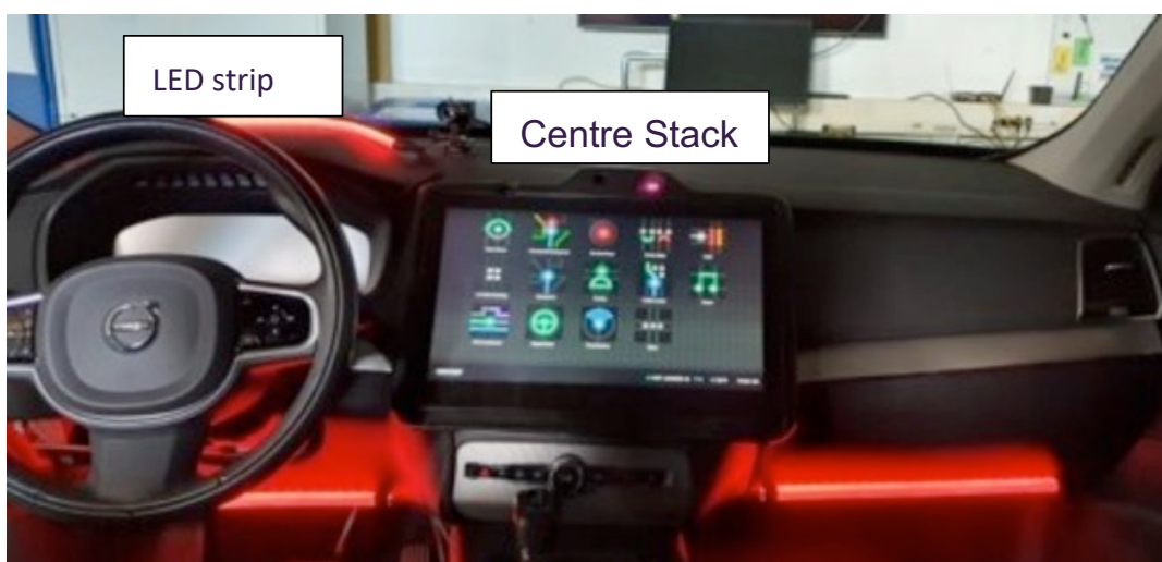
Figure 4.4 LED strips used inside the cabin of the test vehicle to show the driving mode of the TI in-vehicle prototype.
