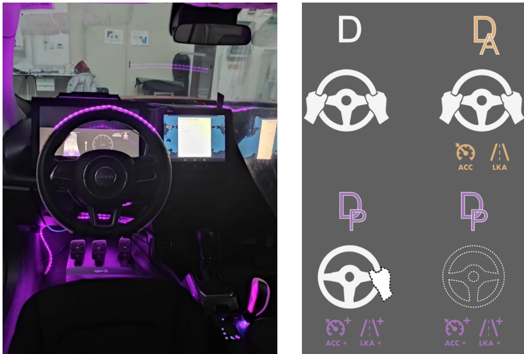
Figure 3.2 LED strips and ambient lights visualizing Driver Standby. To the left is an overview of driving mode icons: Manual (D), Continuous Mediation (Assisted driving, DA), Driver Standby (Piloted driving, DP), and Time to Sleep (Piloted driving, DP).
