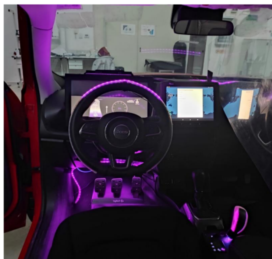
Figure 12 Ambient lighting in Technology Integration Prototype vehicle that was used for on-road evaluation of Mediator system
