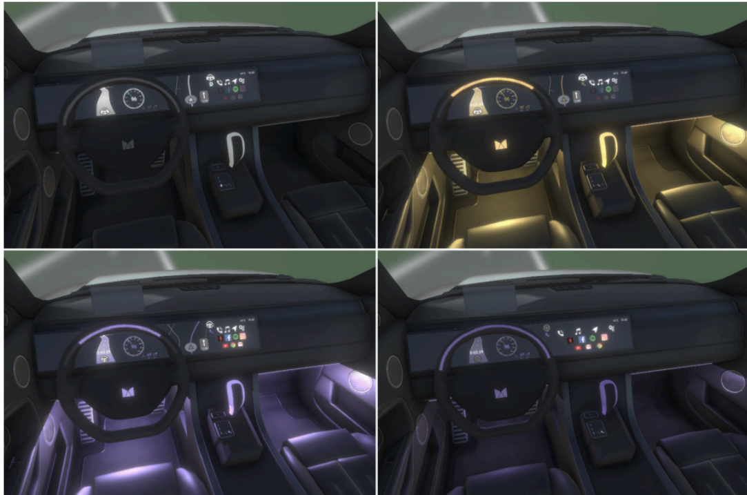
Figure 11 The HMI design in the four different modes: the 'Manual' (M) mode in the upper left picture, 'Continuous Mediation' (CM) in the upper right picture, 'Standby' (SB) in the lower left picture and 'Time-to-Sleep' (TtS) in the lower right picture.
