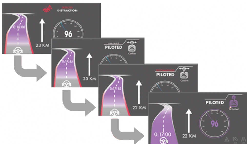
Figure 17 Sequence of displays for suggested mode switch by the Mediator system in case of distraction. To elicit the urgency of the situation the roadsides are turned red.
