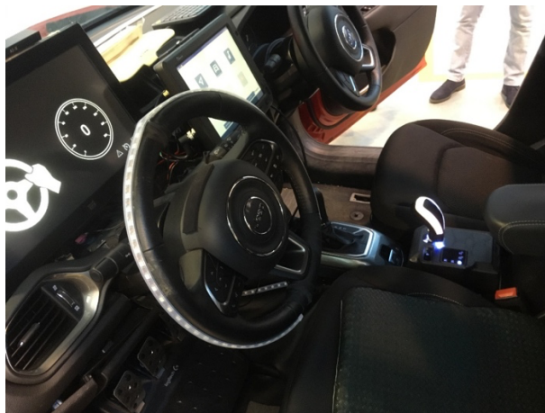
Figure 19 Force feedback shifter in the HF prototype vehicle, placed in the mid console behind the vehicle's original shifter and recognisable by its lighted grip.
