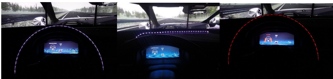
Figure 8 HMI –1 (left), HMI-2 (middle) showing active Piloted mode and HMI-1 (right) showing unplanned takeover request initiation with pulsating red.
