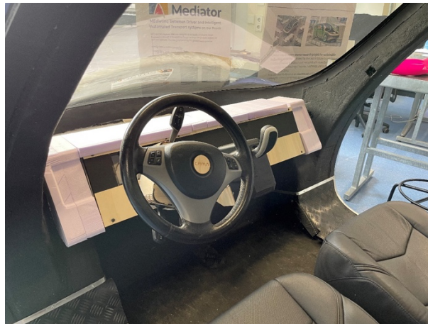
Figure 20 Intended position of the Force Feedback Shifter, next to the steering wheel, in an HMI mock-up.
