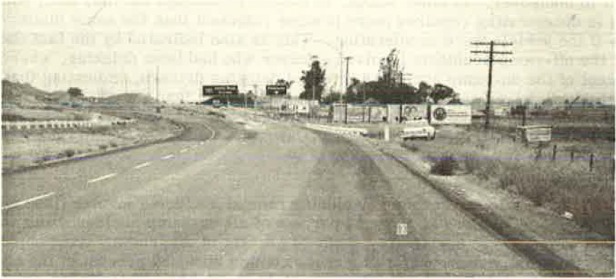
Figure 12. Numerous fixed objects and also the pavement texture and alignment which makes the ramp appear to be the mainline.
