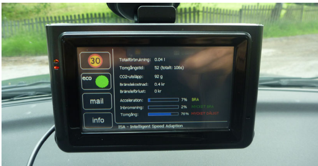
Figure 3 ISA with fuel saving and economical driving functionality
