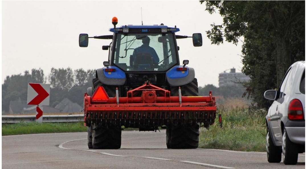
Figure 3. Tractor with tool (harrow), flashing light and at the rear left the retro-reflecting triangle (photo: H. Dijkema).
