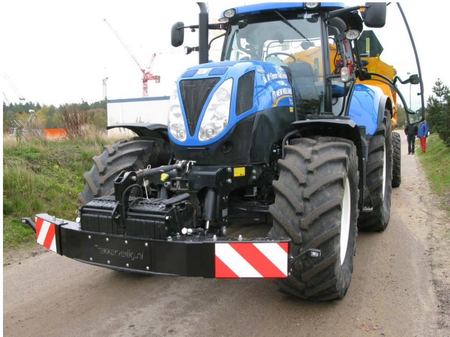
Figure 4. Example of a tractor bumper (photo: SWOV)
