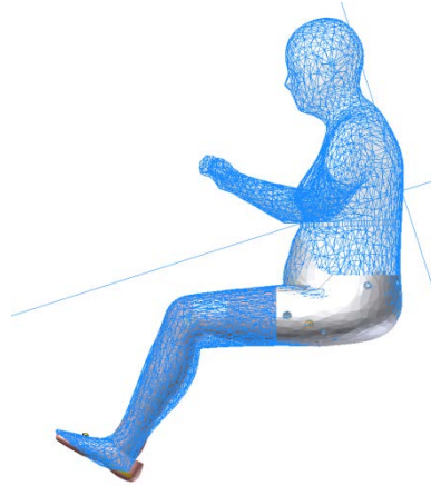
Figure 32: Overlay of 3D UMTRI profile over EATD lower body CAD
