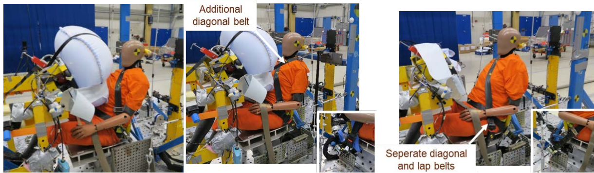
Figure 22: SENIORS buck, EATD 3 point belt left, criss-cross belt centre and split buckle right
