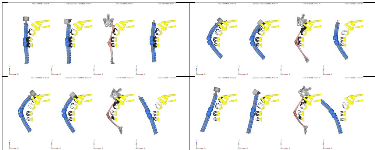
Figure 38: Impact kinematics during simulations against SAE buck (SUV)
