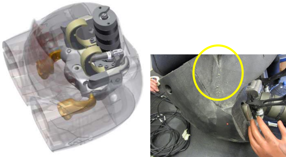
Figure 44: Pelvis area deterioration
