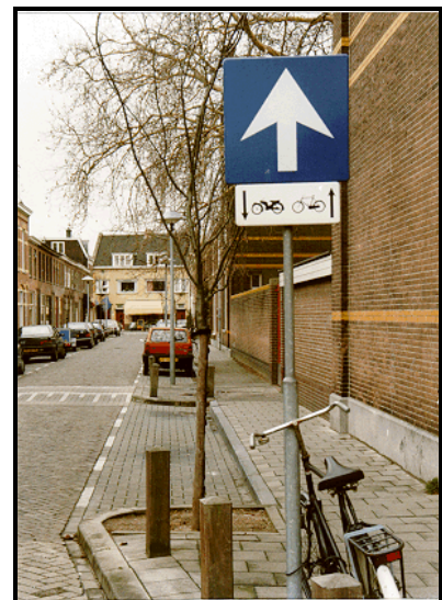
Partial one-way traffic with tight profile Photo: SWOV, Institute for Road Safety Research, A. Vis
