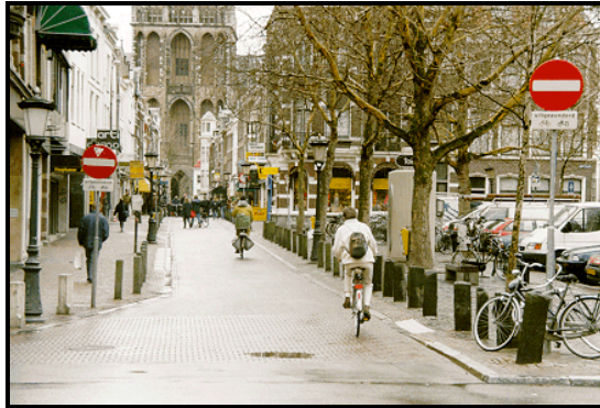
Partial one-way traffic with tight profile Photo: SWOV, Institute for Road Safety Research, A. Vis
