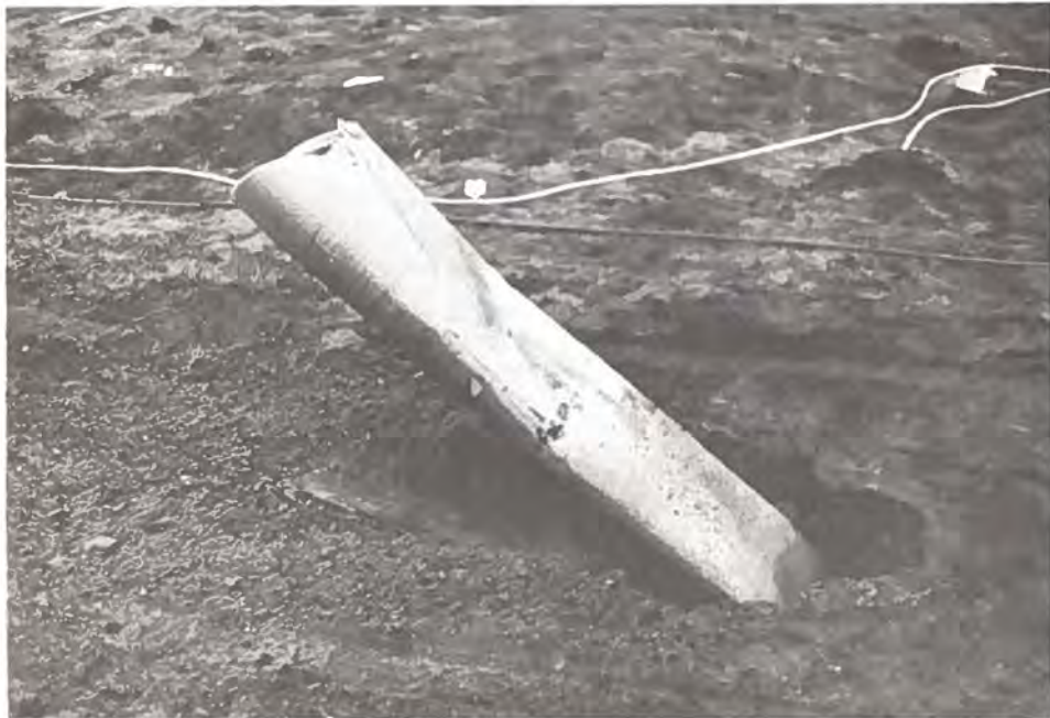
Figure 11. In tests with sand-filled columns the column also broke off at the level of the door opening. The root section however was pulled only slightly out of the ground; it did not break off but folded over at ground level.
