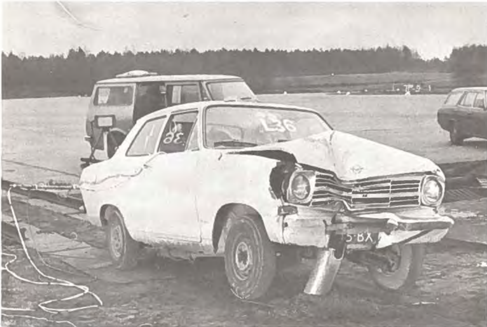
Figure 13. In head-on tests with 10 m aluminium sand filled columns, the root section was only bent over at the height of the cable opening so that the bottom of the column stood upright at an angle. Because of the low impact speed, the vehicle came to a stop against the stump.
