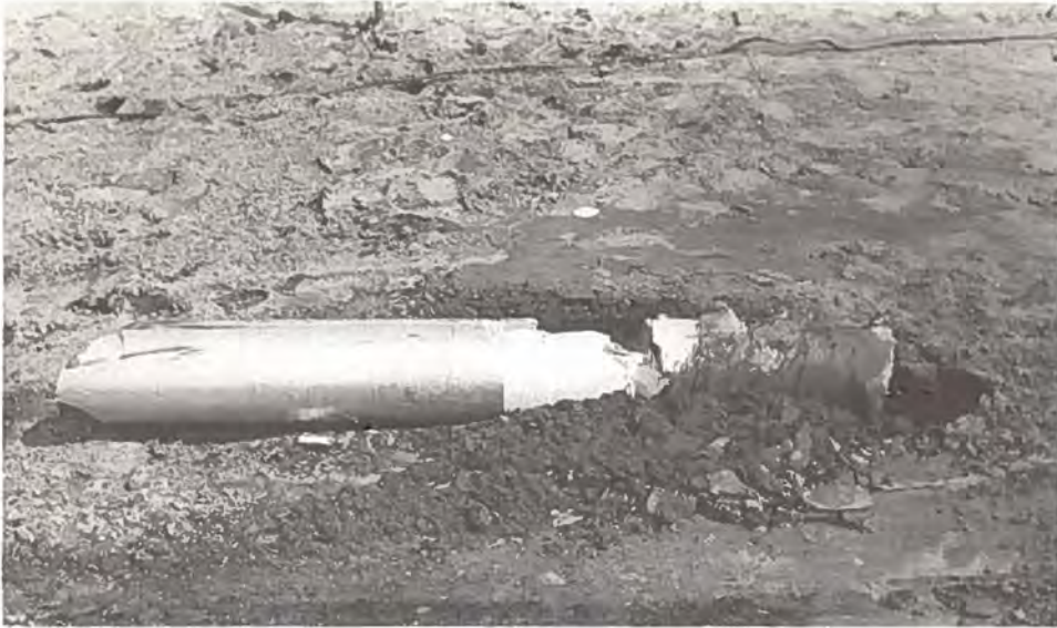
Figure 10. In head-on tests with 10 m aluminium columns not filled with sand the columns broke off at the bottom of the door opening; the root sections were torn about 30 cm out of the ground and broke entirely or partly at the level of the cable opening.
