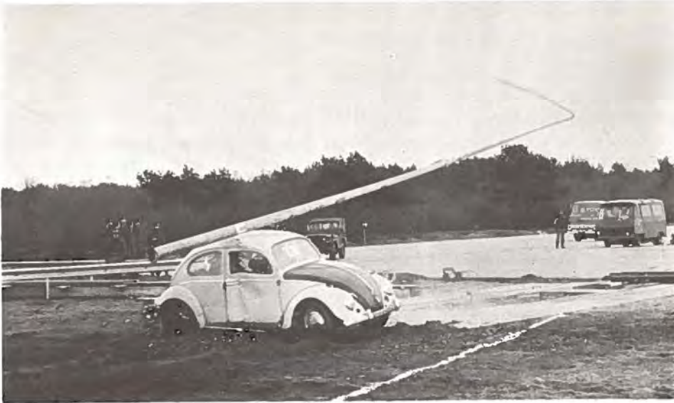
Figure 7. This 10 m slip-design steel column hit laterally in test series B at 42 km/h, gave low vehicle decelerations. It fell on the car's roof; both sideways and roof dents remained within the maxima.
