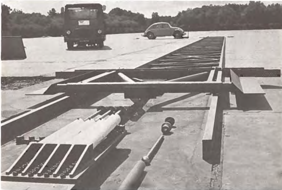
Figure 5. Special equipment was designed for making reproducible sideways ™ on impact tests. The vehicle is placed transversely on a dolly which can be propelled along rails. At the end of the track the dolly is braked suddenly with a braking device, the vehicle slips off the dolly and against the object.
