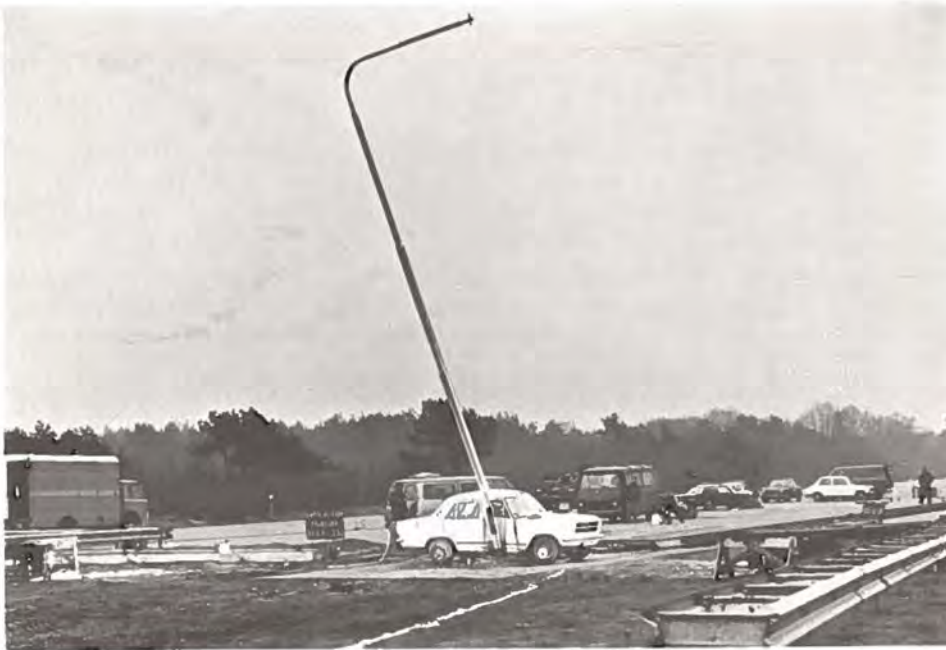
Figure 8. This 10 m aluminium column hit sideways-on in test series C at 30 km/h gave acceptable vehicle decelerations. But it did not break; the vehicle came to a stop against it. The dent in the vehicle's flank exceeded the maximum.
