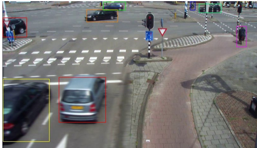
Figure 2.7. Object detection of cars and cyclists (image from TNO)
