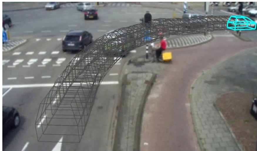
Figure 2.8. Trajectory of identified car over several frames (image from TNO)
