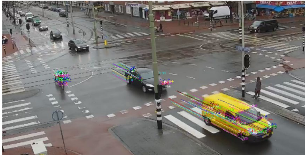
Figure 2.5. Tracked features of two vehicles and one cyclist over several frames
