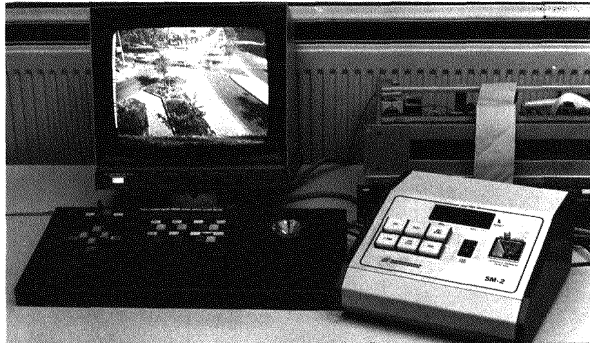
Fig. 5. Monitor, remote-control of the video recorder (at the right) and the special keyboard (black) with 16 programmable push buttons and the control of the electronic crosshairs: a joystick and at the left four pushbuttons.
