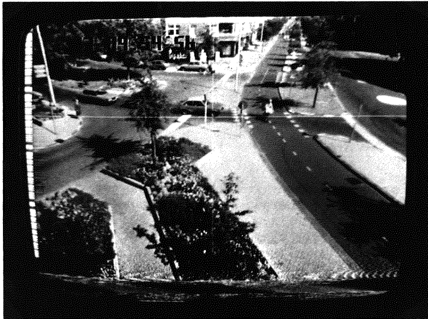
Fig. 3. Video still with digital label at the left, electronic cross-hairs, time and noise bar (at the bottom).
