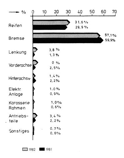
Figure 1. Accident causative defects (Source: DEKRA, 1982)
