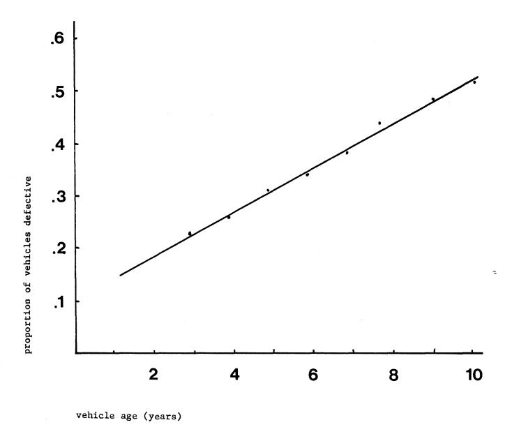
Figure 2. Vehicle age versus defects (Source: Abbene, 1978)
