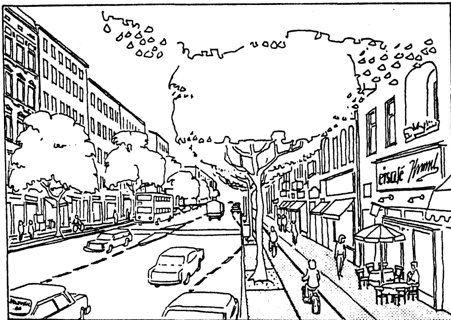
b) second proposal with the old width of driving lanes (11m) and a bike-path on the sidewalk, additional pedestrian crossings and trees
