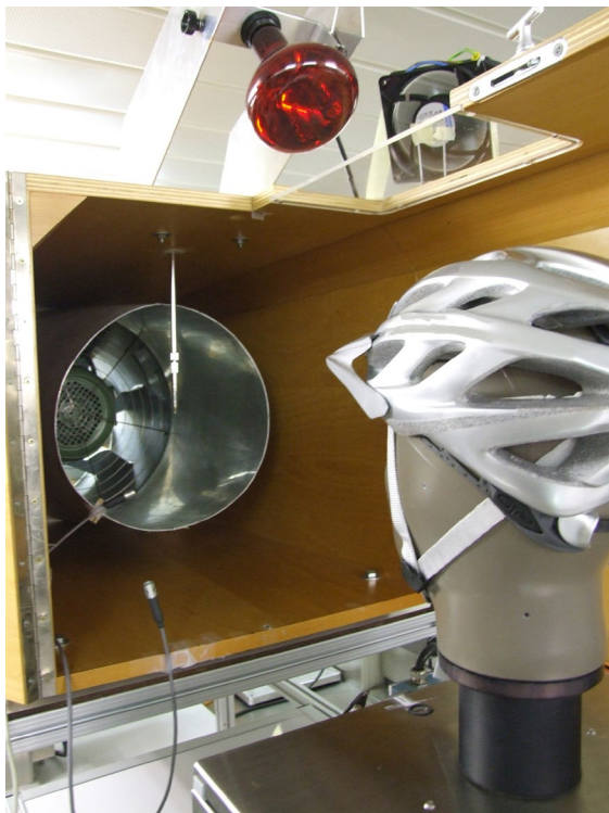
The advanced thermal manikin headform at Empa.
