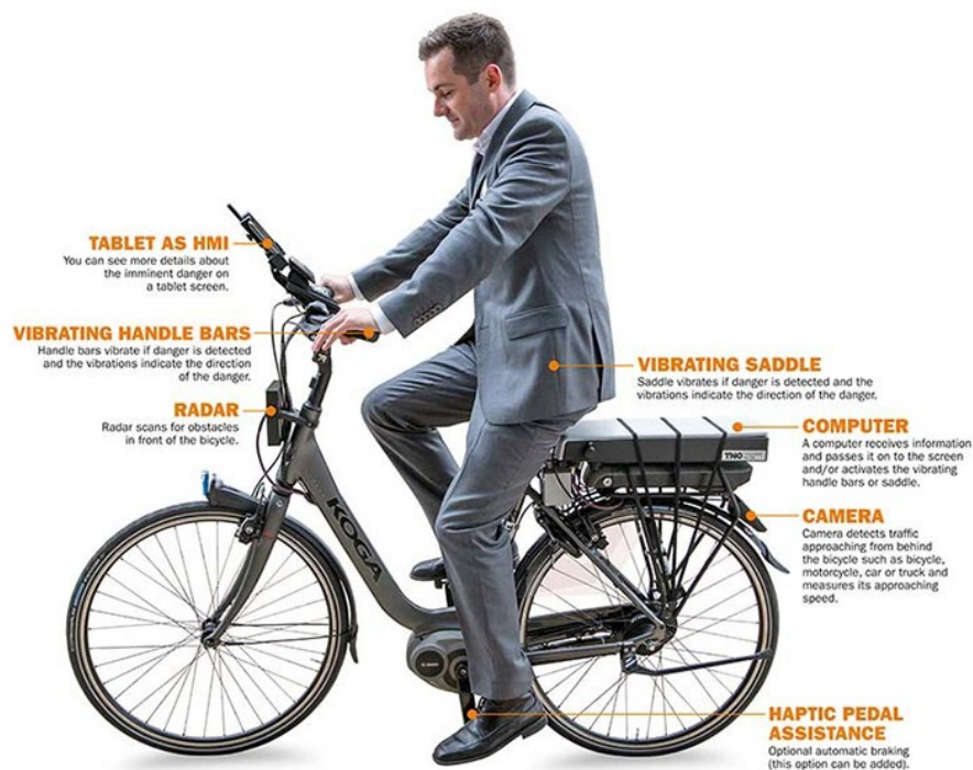
Figure 5. Prototype of the intelligent bicycle, developed by TNO. Source: [54].
