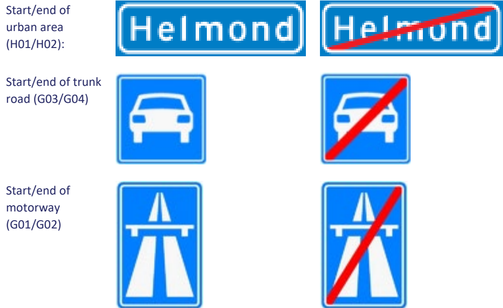
Figure 6. Road signs from which speed information is to be deduced (Source: verkeersbordenoverzicht.nl )
