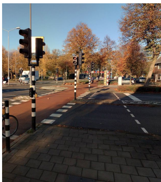
Figure 5. Above: pedestrian light at the beginning of the crossing, the 'Maastricht position' (Photograph: Eric Greweldinger). Below: Before and after installing pedestrian lights at the 'Maastricht position' in the city of Den Bosch (Photograph: Cyclomedia).
