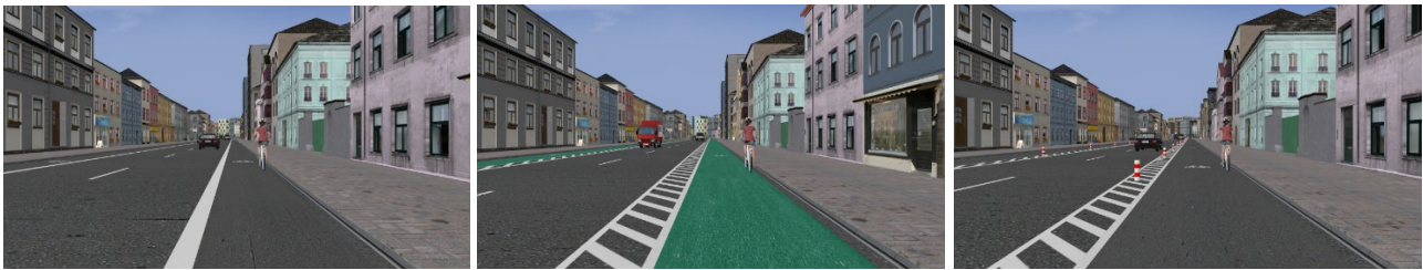
Figure 1: Screenshots of the different scenarios #01 on the left (narrow, wide line making, asphalt grey), #10 in the middle (medium, striped buffer marking, green) and #17 on the right (wide, bollards, asphalt grey).
