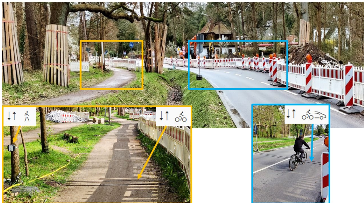
Figure 1 Set-up of the traffic counting system. Yellow - pedestrian and cyclist counting on the sidewalk. Blue - vehicle and cycling counting on the shared lane.
