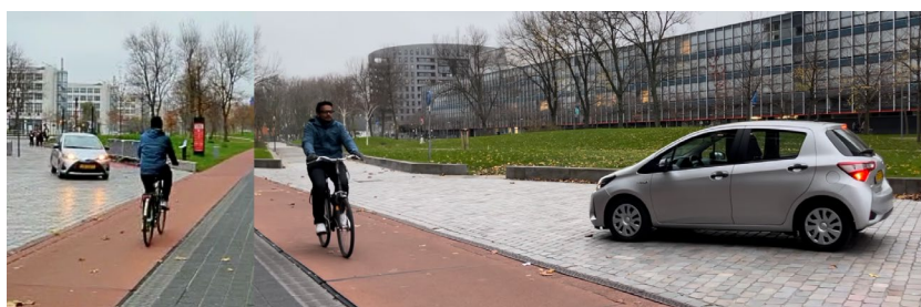
Figure 1: The cyclist participant is cycling straight with the vehicle approaching from their left-hand side. The driver is wearing a seat suit to imitate a driverless vehicle.
