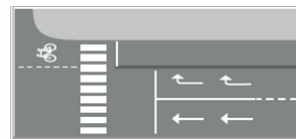
Type 3: Full-length cycle track separate right-turn lane
