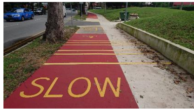
Figure 3: Dedicated cycling path with red segment for AM device
