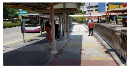
Figure 4: Provision of by-pass behind the bus stop
