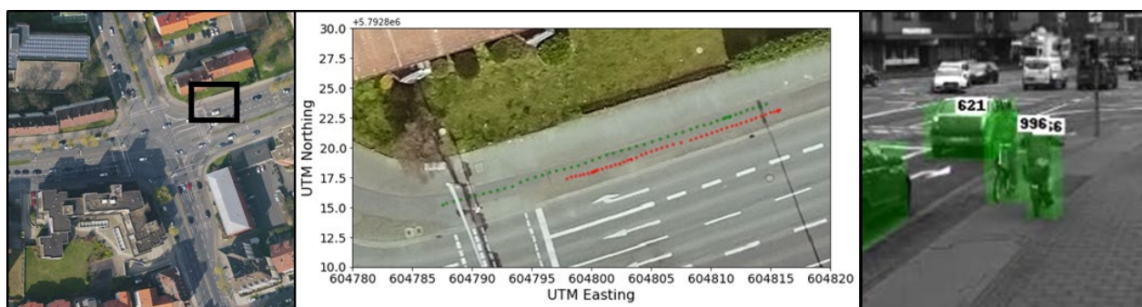
Figure 1: left: Satellite image of AIM Research Intersection (black: area of interest for this analysis); middle: trajectory sample of an interacting bicycle couple in UTM 32U (red: wrong-way cyclists; green: cyclists in the direction of travel); right: video image for this situation
