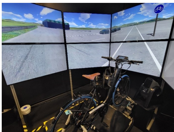
Figure 2: Bicycle simulator and reconstructed test area
