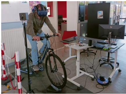
a) VR Bike simulator setup
