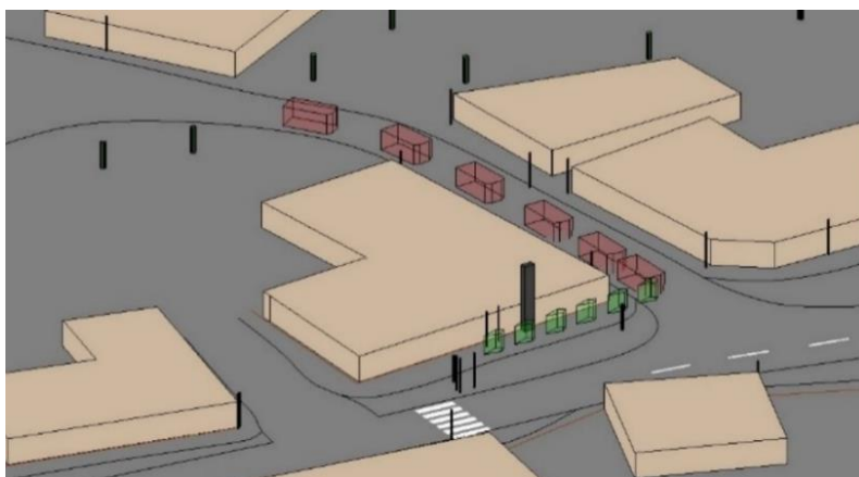
Figure 1: Visualisation of the pre-crash-phase of a crossing bicycle with right of way from bicycle lane right and straight (green – bicycle, red – passenger car, ocher – buildings)
