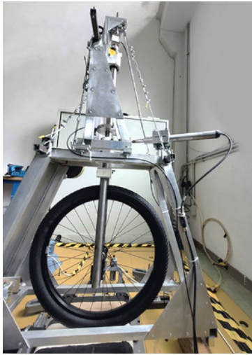
Figure 1: VeTyT test-rig used to measure lateral characteristics of bicycle tyres.
