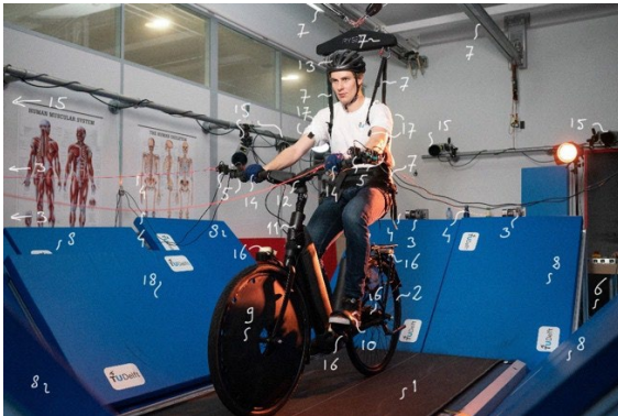
Figure 1. (left) Overview of the experimental setup, with: 1-treadmill, 2-bicycle, 3-pull force motor (4), 4-pull rope (4), 5-force sensor (4), 6-speedgoat real-time controller, 7-intelligent harness, 8-soft padding (8), 9-disc wheel cover (2), 10-foot strap (2), 11-mechanical rotation limiter, 12-rear-brake handle, 13-helmet, 14-protective gloves (2), 15-motion capture camera (12), 16-IMU (4), 17-EMG measurement unit (4), 18-folding fence, and (right) threshold value for the steer impulse perturbation for which the cyclist (45 year, average skill) will not fall as a function of forward speed, the solid line is the mechanics model, the dashed line is the statistical model with a 50 % change of not falling, the dotted lines are the 66 % and 34 % boundaries.
