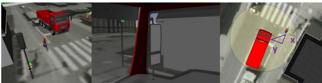
Figure 1: Junction accident with turning to right HGV crossing the bicycle' path (left: front overview; mid: driver's view and obstructed cyclist due to A-pillar; right: top view of the accident scene and the sketch of an ADAS system view)
